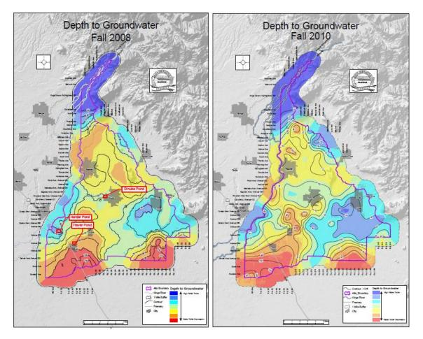
Figure 4a and 4b. Depth to groundwater in Alta Irrigation District, Fall 2008 and Fall 2010 (Alta Irrigation District 2010)
